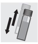
Shake the cell. Undissolved powder has no adverse effect on measurement.
