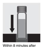
the last reagent was added: Insert the cell in the photometer cell shaft and start measurement.
