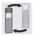
Mix the contents by carefully swaying the cell (10 x / for approx. 30 s altogether).
