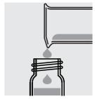
Fill an empty cell with the prepared sample and close it with the screw cap.
