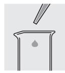
Pipette 25.0 ml of sample into an empty beaker.
