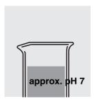
Check the pH value of the sample. Nominal value: approx. pH 7. Correct with diluted sodium hydroxide solution or nitric acid as necessary.
