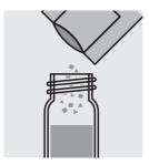
Add the contents of a **VARIO Sodium** Periodate F10 powder pack and close the cell with the screw cap.
