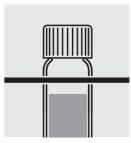
Remove the cell from the thermoreactor and let it cool down in a cell rack.
