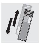
Shake the cell for 10 to 15 seconds. Undissolved powder has no adverse effect on measurement.
