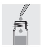
With a pipette add 2.0 ml Vario Sodium hydroxide 1.54N, close the cell with the screw cap and mix.
