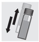
Shake the cell for 10-15 s. A small amount of solid matter remains undissolved.
