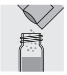
Add the contents of a **Vario Ascorbic Acid** powder packet and close the cell with the screw cap.
