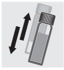
To dissolve solids, shake the cell for approx. 10 to 15 seconds. A small amount of solids may remain undissolved.
