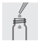
Pipette 10.0 ml of sample into the empty cell.
