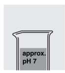
Check the pH value of the sample. Desired value: approx. pH 7. Correct with diluted sodium hydroxide
