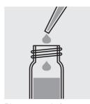
Pipette 2.0 ml of prepared sample into a TN Acid LR/HR (Reagent C) reaction cell and close the cell with the screw cap.
