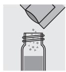
Add the contents of a Vario Monochlor F RGT powder pack and close the cell with the screw cap.
