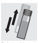
Shake the cell vigorously to dissolve solids. A small amount of solids may remain undissolved.
