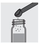
Add 1 level blue microspoon of **N-3K** into a <u>reaction cell</u> and close the cell with the screw cap.
