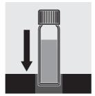
Insert the **16 mm** cell in the photometer cell shaft and start measurement.
