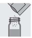
Add the contents of a **VARIO Iron TPTZ F10** powder pack and close the cell with the screw cap.
