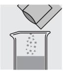
Add the contents of a VARIO SO4-1 TP Sulfa 4 F25 ml powder pack and dissolve them by stirring.
