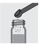
Add 1 level black measuring spoon no. 8 of **Nitrit-101** and close the cell with the screw cap.
