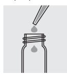
Pipette 10.0 ml of sample into the empty cell.
