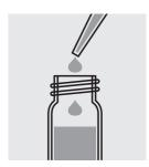
Add 15 drops of Vario Alkaline-Cyanide Reagent Solution and close the cell with the screw cap.
