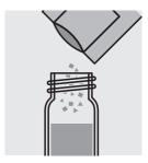
Add the contents of a VARIO Silica Citric Acid F10 powder pack and close the cell with the screw cap.
