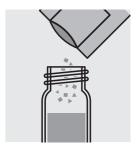
Add the contents of a **VARIO Hexamine F20** powder pack and close the cell with the screw cap.
