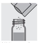
Add the contents of a Vario Phosphate RGT F10 ml powder packet and close the cell with the screw cap.
