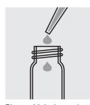
Pipette 20.0ml sample into the empty cell.
