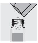
Add the contents of a VARIO AMMONIA Cyanurate F5 powder pack and close the cell with the screw cap.
