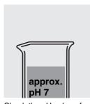
Check the pH value of the sample. Desired value: approx. pH 7. Correct with diluted sodium hydroxide solution or hydrochloric acid as necessary.
