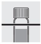
Remove the cell from the thermoreactor and let it cool down in a cell rack.
