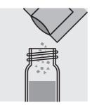
Add the contents of a **VARIO Aluminum** ECR F20 powder pack and close the cell with the screw cap.
