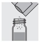
Add the contents of a **MolyVer 3 Reagenz** powder pack and close the cell with the screw cap.
